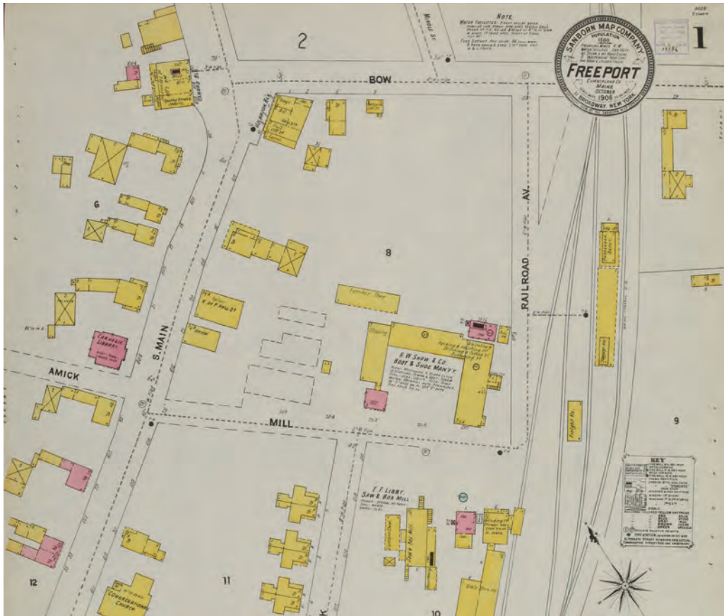
Fire insurance map of Freeport Village 1906. The Sanborn Map Company of Pelham, NY published detailed insurance maps of cities and towns that were used by insurance companies to insure buildings they had never physically seen. The information contained on these maps includes street name and number, building construction type, occupancy, and fire protection such as sprinkler systems. They were used extensively from the 1860s to the 1960s.
